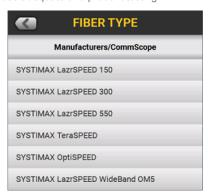
Figure 5. CertiFiber Pro supports all SYSTIMAX High Speed Migration fiber types
