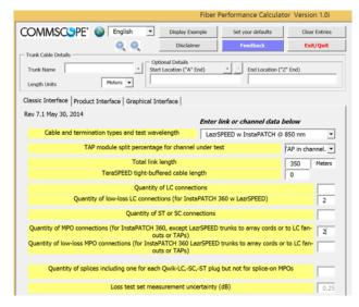
Figure 2. CommScope Link Loss Calculator for SYSTIMAX fiber installations.
