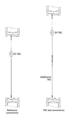
Figure 6. Reference and TRC Test Connections for Far End Source Mode
