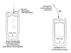
Figure 8. Connections for Testing the Tap Port Links from the Near End through an EDGE Module
