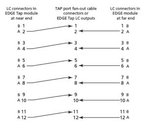
Figure 5. Connections from the Near and Far End Modules to the TAP Port Cable
