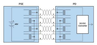
All four pairs are used to deliver power in an IEEE 802.3bt PoE system, power is transmitted simultaneously with data and is compatible with 10/100/1000/10GBase-T.
