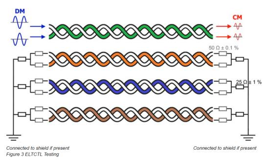
While TCL and ELTCTL parameters are excellent indicators of the balance of a twisted-pair cable, neither is currently a field test requirement under ANTI/TIA-568.C.2 standards. This is because most field test equipment has only been capable of differential mode measurements. TCL and ELTCTL testing have therefore been limited to laboratory environments by manufacturers who must ensure good pair balance characteristics to comply with TIA and ISO/IEC industry performance standards.
