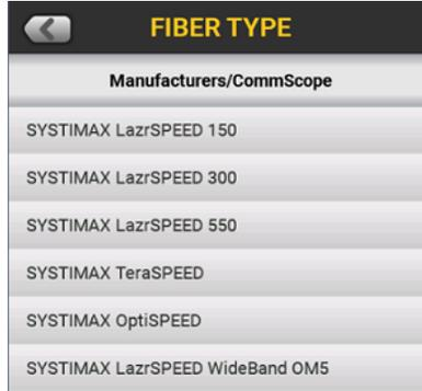
Figure 5. CertiFiber Pro supports all SYSTIMAX High Speed Migration fiber types
