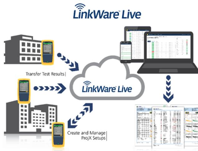
Figure 4. With LinkWare Live, Project Managers can create and manage test settings and transfer them to testers. Techs can upload test results, allowing the Project Managers to track job progress.
