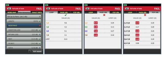
The field testing standard for ANSI/TIA 1152 now includes DC Resistance Unbalance as a field test. Limits are included in ANSI/TIA -568-C.2. It is not a mandatory certification requirement, it is easy to include if you have a capable cable tester like the DSX-CableAnalyzer. But there's a catch. While ISO/IEC 11801 ed. 2.2 provides DC Resistance Unbalance test limits for the Channel and Permanent Link definitions, ANSI/TIA-568-C.2 only provides test limits for the Channel definition.
